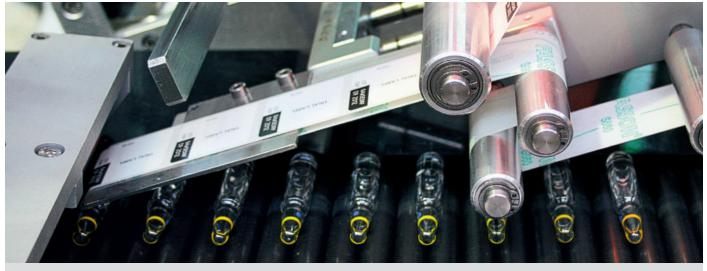
Figure 2: Ampoule Labeler (Labeler Model RML)
