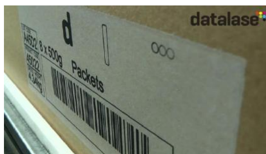
Laser marking directly onto cardboard package
