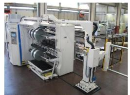
TB-3 remains in the production program and is utilised i.e. when unwind roll diameter is > 1000 mm
