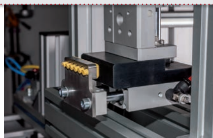
Combination of guide block and dual-piston cylinder
