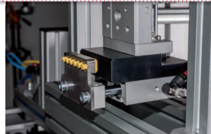
Combination of guide block and dual-piston cylinder
