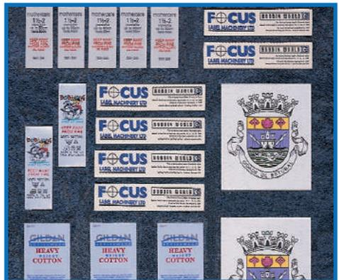
In all cases with textile labels, the finished printed products will need to be cured in an industrial oven at 125 degrees centigrade for approximately two hours. This fixes the ink to the substrate to maximise its longevity and ensure uniform quality across the batch.
