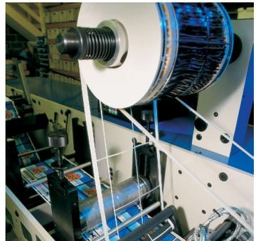
**Outfeed and Rewind:** The output section maintains tension as the substrate leaves the printing press, by means of tension control sensors. Waste products are rewound out of the system and the final products are rewound into large rolls for later inspection.
