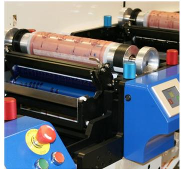
**Drying Station:** each colour should be dry before the next is applied to the substrate. The drying section might include a combination of Infrared & Air drying or UV / LED curing or both systems. Better machines will ensure the drying intensity is matched to the press speed which can be variable with different applications.
