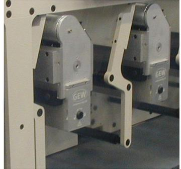
**Die Cutting & Converting:** these are more commonly found on narrow web presses for production of labels, tickets & cartons. Products can be cut, creased, Foiled, Stamped, Embossed, perforated all in line in the same operation as printing. Therefore producing the finished product or label in roll or sheet form. Die cutting modules need to be built with heavy duty components for the high levels of pressure/force required to convert flexible webs up to 300gsm.
