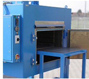
ovens with charging trolleys / Herdwagenöfen
