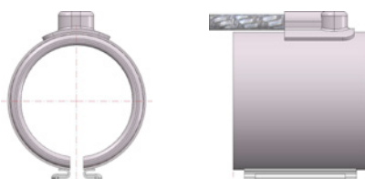
axial flat cap, only with DGM/DAK/DMK Flachkappe axial, nur bei DGM/DAK/DMK
