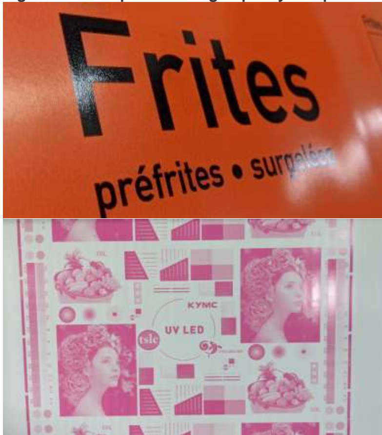
Figure 1 : Solid print with high opacity and providing a lifted relief touch
