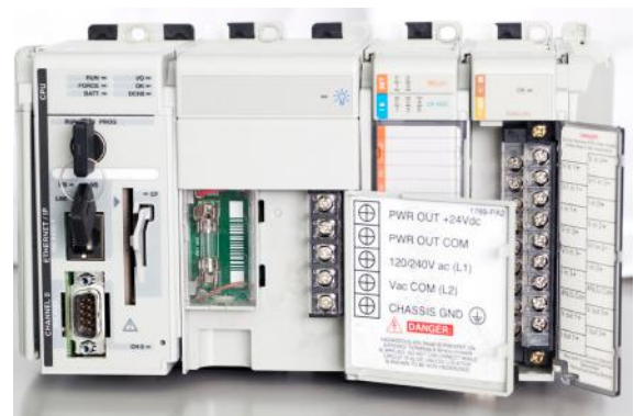
Figure 16: A programmable logic controller (PLC) that networks local devices over EtherNet/IP.
