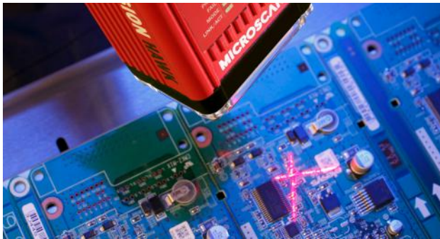
Figure 9: A barcode reader decodes a symbol on a PCB to acquire part data and log the part as it enters the assembly process.
