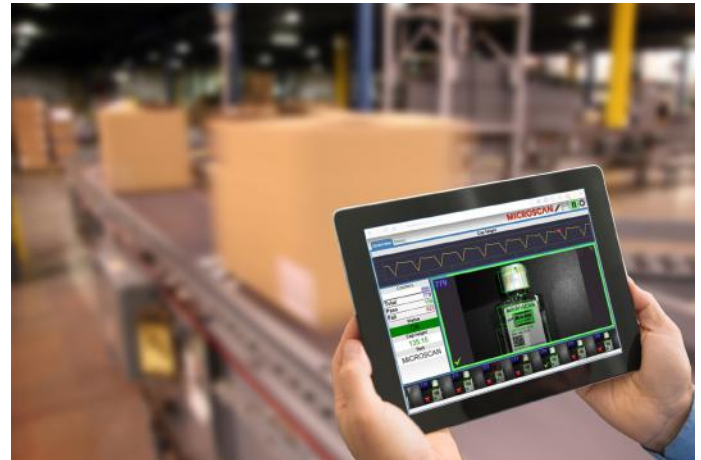
Figure 6: A web user interface displays inspection data from a machine vision system on the factory floor, allowing inspections to be monitored through a web browser on any local device.
