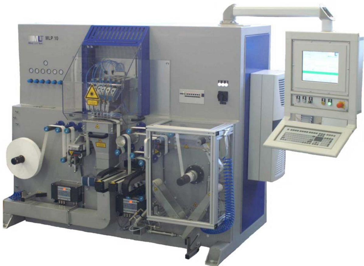
Picture shows the turnkey MLP-10 system including the Micro Perforator, the Rewinder, the CO 2 - Laser Source.
