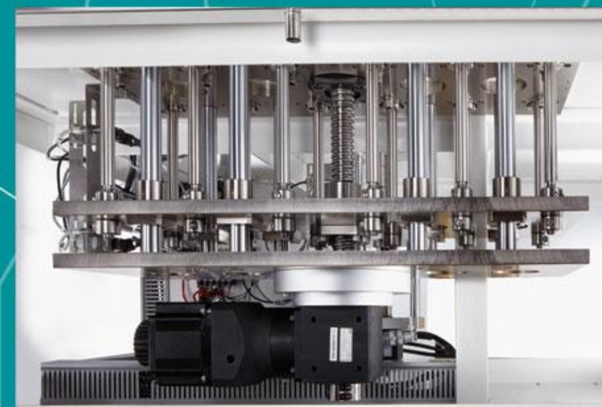
Servo driven vertical piston stroke for absolute reliable accuracy.
