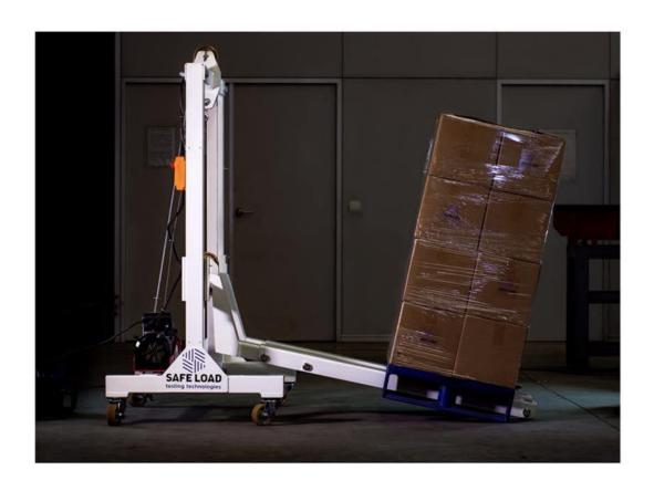
Tilt testing was conceived as a method to evaluate the resistance of load securing systems. In this case, the force of gravity is used to replicate its effect during transportation and study the load's stability in this situation.
