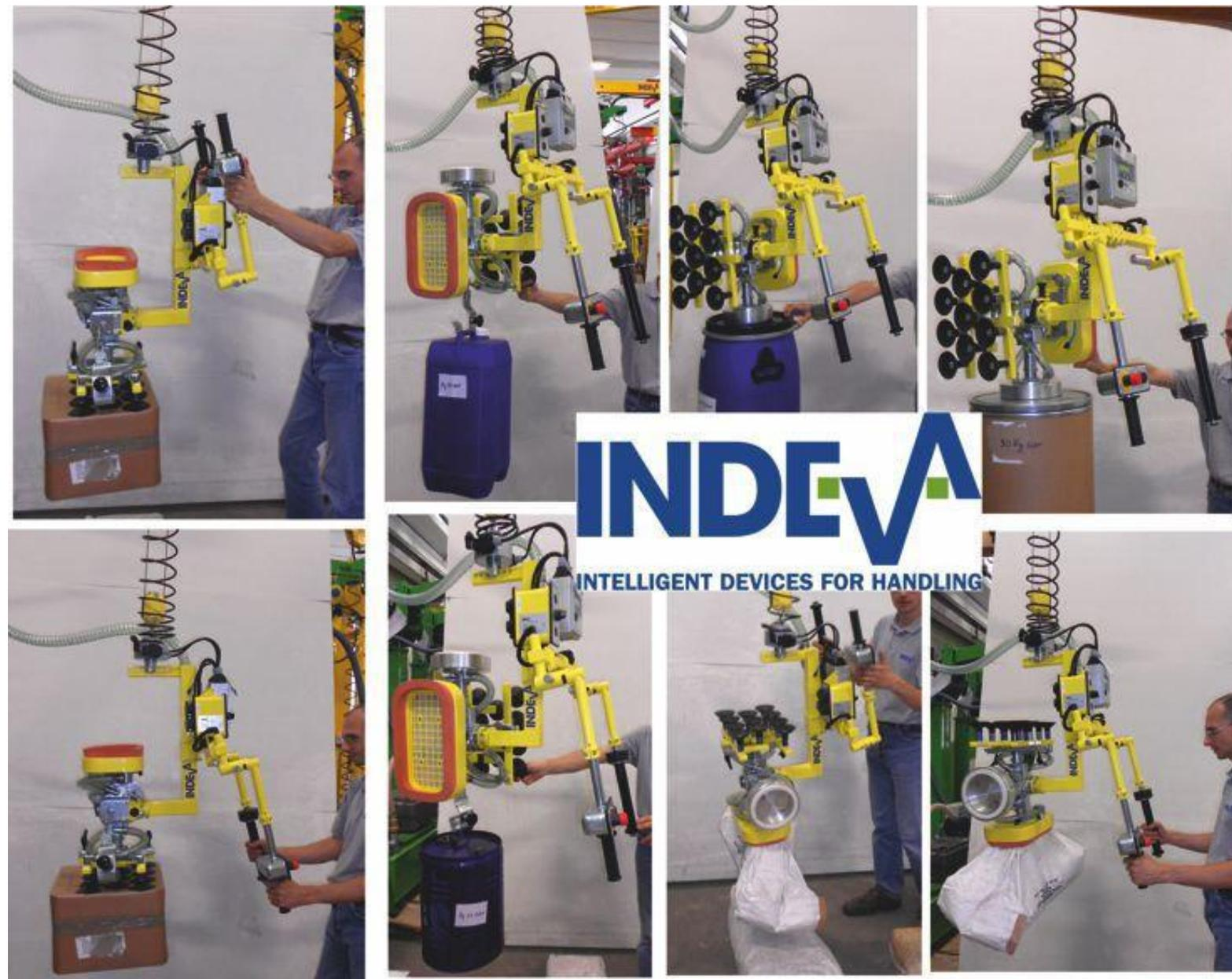
This INDEVA, Liftronic model, could fully satisfy this Company' request for a lift assist device for the operator that has to lift 4 different types of load in a quick yet precise and ergonomic way, repetitively during his whole work shift.
