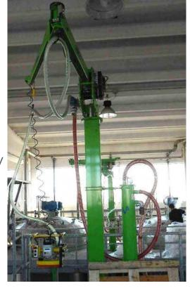
This allows the operator to work with lots of bags of different weights without having to adjust the system to the new weight or to pre-select a different setting each time.
