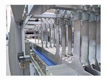
Rounded safety doors, which increase the space inside the machine frame and ensure:
