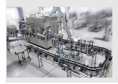
From a mostly manual to an automatic production is only a short step, thanks to the new turn-key line provided by ENOBERG, that includes: a rotary monobloc from the ELC 12-12-1 B A series; a rotary table to manually upload bottles; inspection systems for the checking the the presence and correct position of the cap; a progressive expeller to expel any non-compliant bottles and asaturator to carbonate the water.
