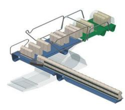
With the single lane infeed, it is possible to work lots of different kinds of containers, with different sizes, without having to have additional belt equipment. Therefore, format changeover is much faster and easier, as there is no need to regulate the guides on the different lanes.
