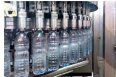
The 12,000 bottles per hour bottling line installed in the plant in Zhdanovichi makes use of a latest generation automation and control system called VaryLine System® that, together with the use of sophisticated sensors, allows you to maintain high levels of operational efficiency throughout the production cycle, thus reducing costs and energy consumption.
