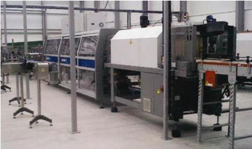
6 oz. tinplate cans in 1x3 and 1x2 collations. The machine chosen by Hida is very versatile and can also pack bottles, cartons and plastic, metal and glass jars in various types of pack at speeds up to 300 pack/minute (depending on the type of container and format selected).
