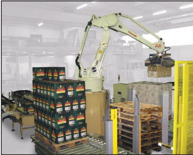
Gripper pick up system with suction cups for cartons.
