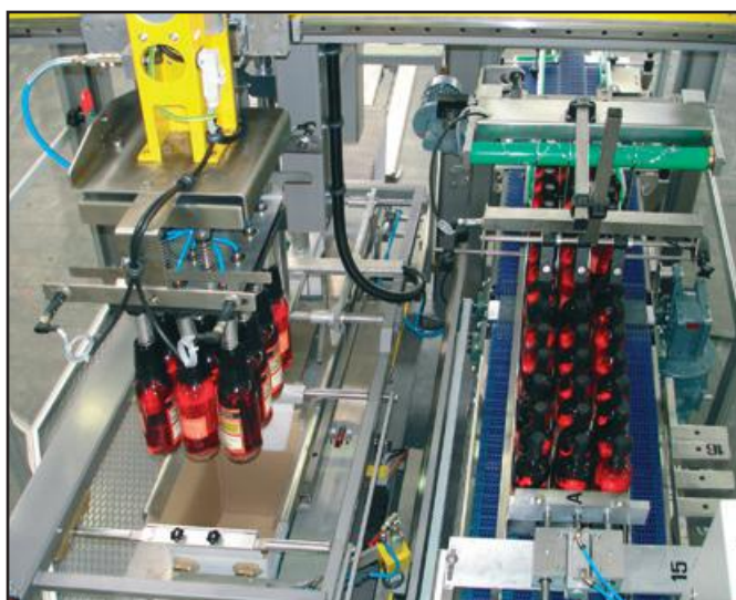
Bottles cartoning machine with bells pick-up head system.
