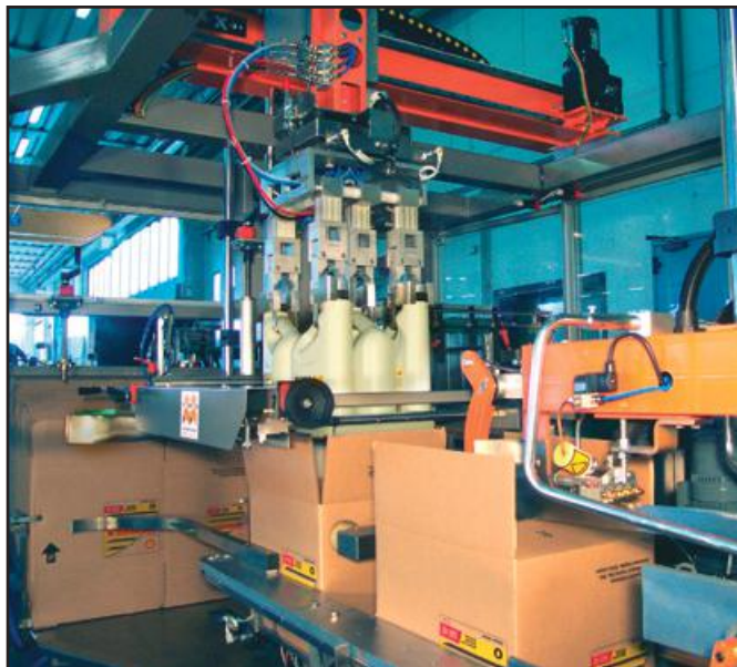
Carton erector, carton packer and carton sealing with hot melt glue.
