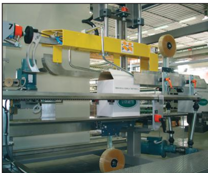
Carton closing and sealing machine with adhesive tape.
