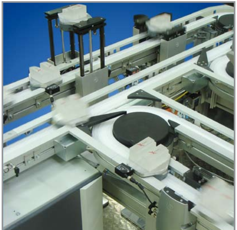
Individual work stations for manual or automatic operations, testing etc can easily be added to a line.
