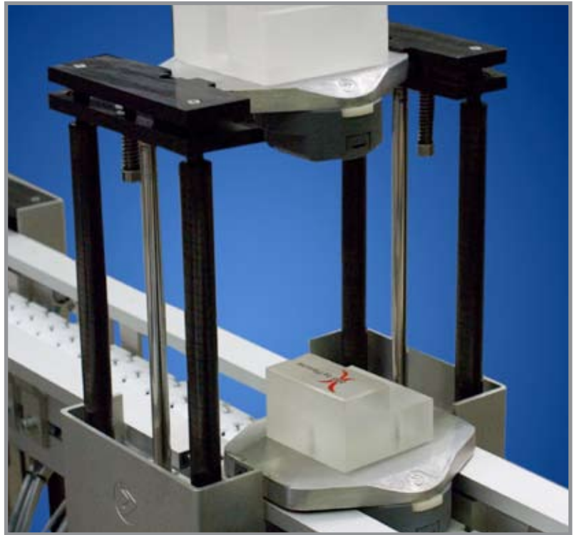
Tunnel locating modules can in pair serve one robot or machine enable continuous operation – highest possible utilization of the equipment.
