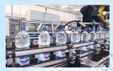
he 12,000 bottles per hour bottling line installed in the
