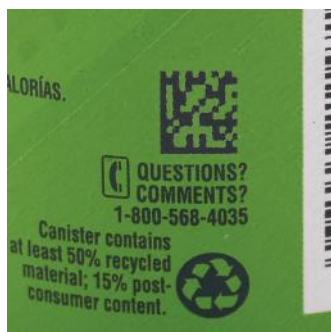
Figure 10: During the design of this label, the original Data Matrix code was stretched and resized. These changes may result in readability and compliance issues down the line.
