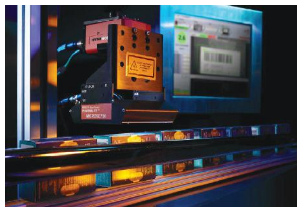
Figure 6: A verification system installed on the packaging line uses a unique camera-and-lighting configuration to capture images of labels, which are verified for ISO/IEC print quality by machine vision inspection software.
