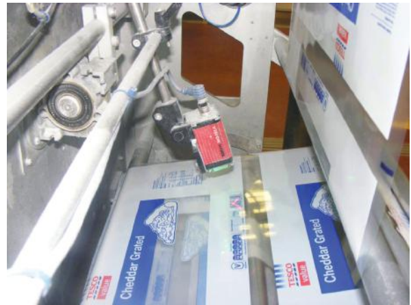
Figure 15: Harsh manufacturing conditions may result in damage to high-quality labels in production, so it is important to re-verify labels after any operational stage where damage is likely.
