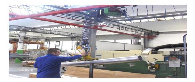
The INDEVA manipulator reacts in real time with no inertia forces when reversing load direction, saving your operators from the damaging physical strain these direction changes can have on their bodies. Lifting operations with an INDEVA are really ergonomic and effortless for the operator.
