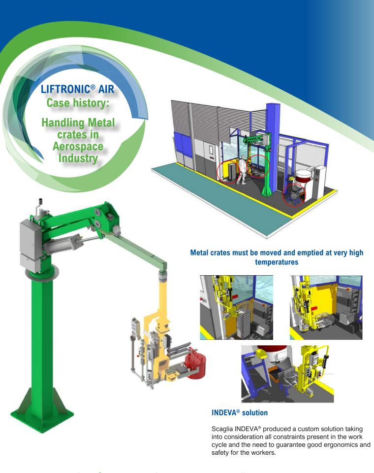
A column mounted Liftronic® Air with tooling for handling and rotating offset crates.
